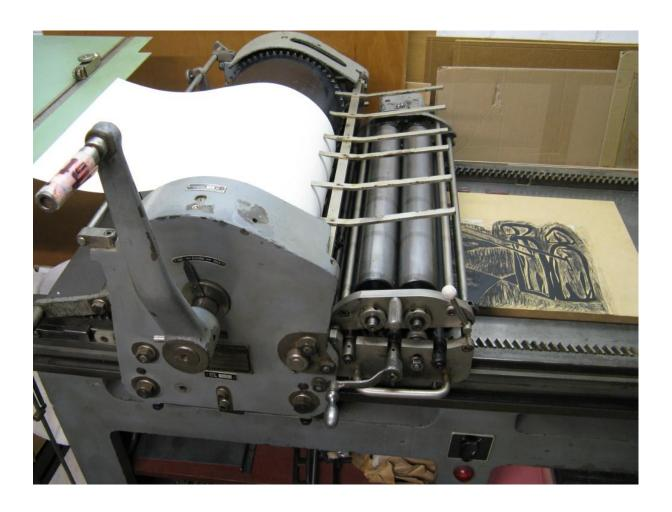
A sheet of paper is picked up by the printing cylinder and rolls over the wooden block. The ink-covered rollers are leaving ink upon the flat surface but not in the non-printing areas.
